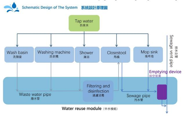
The modularized indoor reclaimed water integration system is an original technology, which is a new technology for indoor water saving and reusing in buildings.
