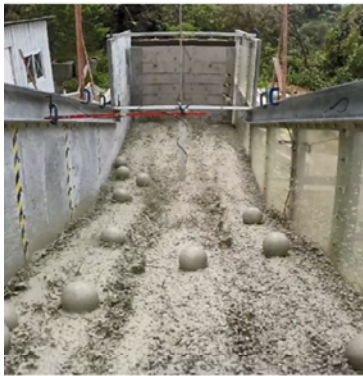
Testing of Debris Impact (泥石流撞擊試驗)
