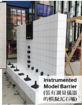
Testing of Boulder Impact (大石撞擊試驗)
